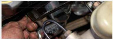
On driver side, remove dipstick and tube. Bend the front brake line slightly forward and you'll have enough room to remove tube.
