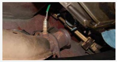
Remove the nuts at the collectors for the mid-pipe and drop the mid-pipe down and back, out of the way.
