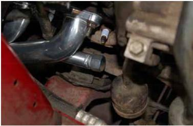
Install the provided steel caps on front EGR ports if not used. If used, connect the tubes.
