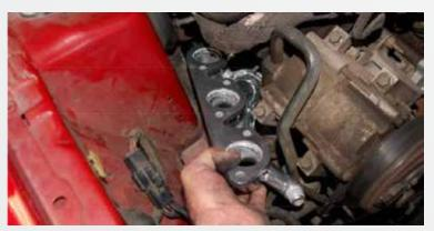
Remove nuts and studs and stock manifolds from both sides. The manifolds will come out from the top. Passenger side installs from the top and driver side from below. Fig. 4 and 5  $\,$
